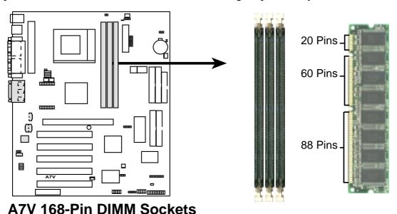
The DIMMs must be 3.3Volt unbuffered SDRAMs. To determine the DIMM type,
