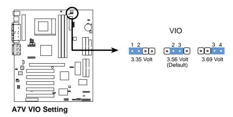
**WARNING!** Using a higher voltage may help when overclocking but may result in the shortening of your computer component's life. It is strongly recommended that you leave this setting on its default.
