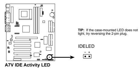
**NOTE:** The LED *will not* light up during read and write activity by devices connected to the Primary or Secondary IDE connectors of motherboards with PCB versions earlier than Rev. 1.01.P (for example, Rev. 1.01.). To check your PCB version, see the area between PCI4 and PCI5 and look for the marking that starts with "REV."
