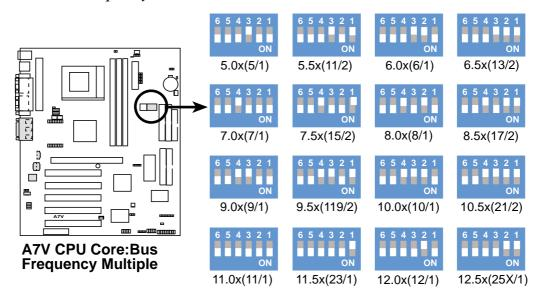
**NOTE:** If your processor does not have a locked Frequency Multiple, you must use **CPU Core:Bus Freq. Multiple** to set the Frequency Multiple. If the Frequency Multiple of your processor is locked, setting the Frequency Multiple will have no effect.
