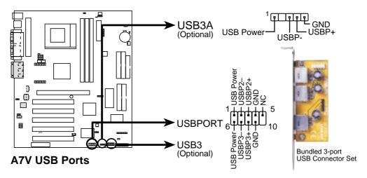
Recommended Setup: Use USBPORT + USB3A with the bundled 3-port connector set.
