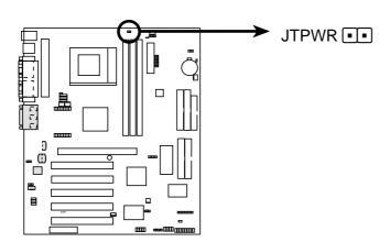
A7V Power Supply Thermal Sensor Connector
