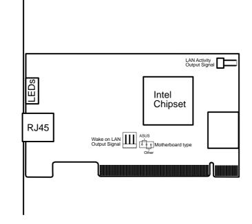
If you are using the ASUS PCI-L101 on an ASUS motherboard, leave the jumper on its defaut setting of "ASUS." If you are using another brand of motherboard, set the jumper to "Other." Connect the Wake on LAN (WOL) output signal to the motherboard's WOL\_CON in order to utilize the wake on LAN feature of the motherboard. Connect the LAN activity output signal (LAN\_LED) to the system cabinet's front panel LAN\_LED in order to display the LAN data activity.
