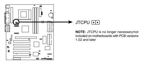
**A7V CPU Thermal Sensor Connector**
