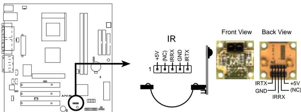
**A7V-M Infrared Module Connector**
