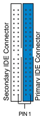
**NOTE:** Orient the red markings (usually zigzag) on the IDE ribbon cable to PIN 1.
