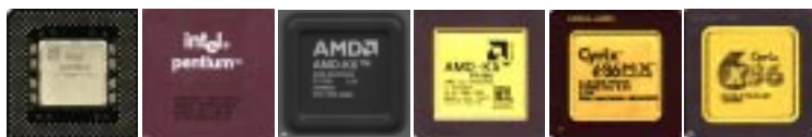
Pentium MMX (P55C) (150MHz-233MHz) Intel Pentium (P54C) (75MHz-200MHz) AMD-K6 (PR166 and faster) AMD-K5 (PR75-PR133) IBM/Cyrix 6x86(MX) (PR166 and faster) IBM/Cyrix 6x86(M1) (PR166 and faster)
