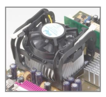
Figure 2-11 Fan and Retention Mechanism Installed and Locked
