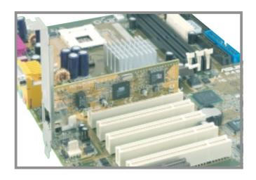
Figure 2-18 Installed PCI Card
