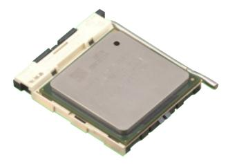
Figure 2-8 Installed CPU
