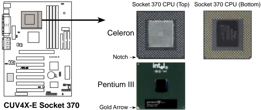
Note in the illustration that CPUs have marks (usually a notch or a gold mark on one corner) to help you identify the proper orientation and enable you to correctly install a CPU. It is important that you match the marked corner of the CPU with the corresponding corner on the socket so as not to damage the CPU pins.
