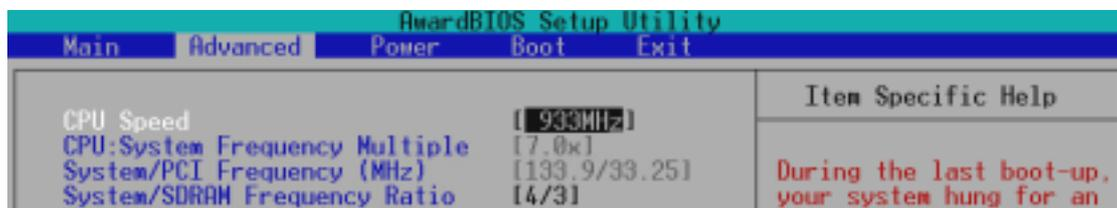
**Cause for Hangup: Improper CPU Speed**
