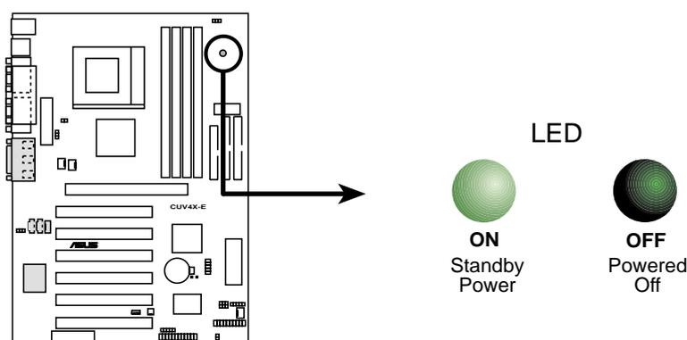
CUV4X-E Onboard LED
