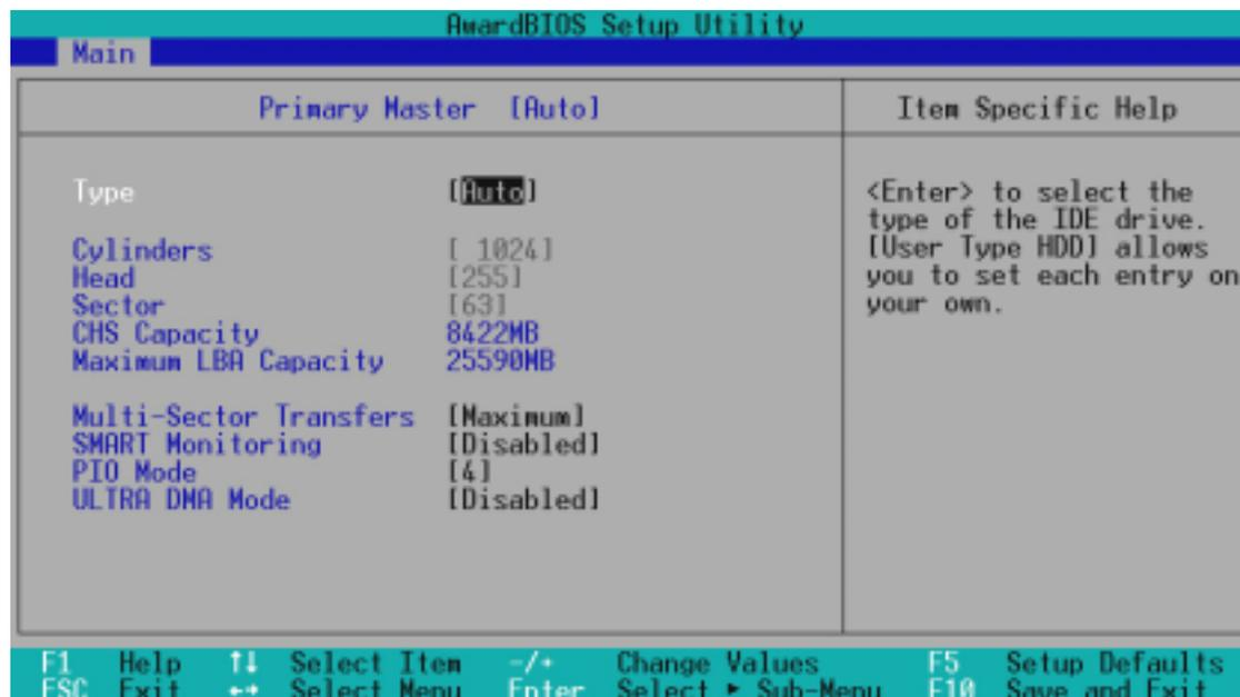
**NOTE:** Before attempting to configure a hard disk drive, make sure you have the configuration information supplied by the drive manufacturer. Incorrect settings may cause the system to fail to recognize the installed hard disk. To allow the BIOS to detect the drive type automatically, select [Auto].
