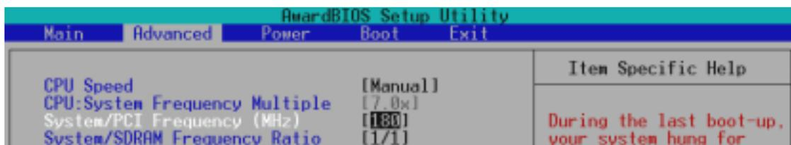
**Cause for Hangup: Improper System/SDRAM Frequency**
