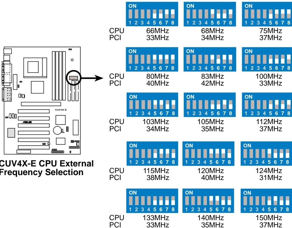
**WARNING!** Set the CPU frequency only to the recommended settings. Frequencies other than the recommended CPU bus frequencies are not guaranteed to be stable. Overclocking the processor is not recommended. It may result in a slower speed.
