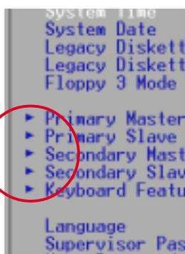
Note that a right pointer symbol (as shown in the left view) appears to the left of certain fields. This pointer indicates that you can display a sub-menu from this field. A sub-menu contains additional options for a field parameter. To display a sub-menu, move the highlight to the field and press <Enter>. The sub-menu appears. Use the legend keys to enter values and move from field to field within a sub-menu as you would within a menu. Use the <Esc> key to return to the main menu.
