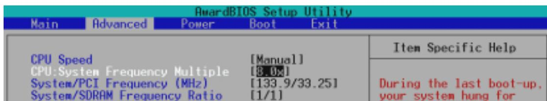
**Cause for Hangup: Improper CPU: System Frequency Multiple
