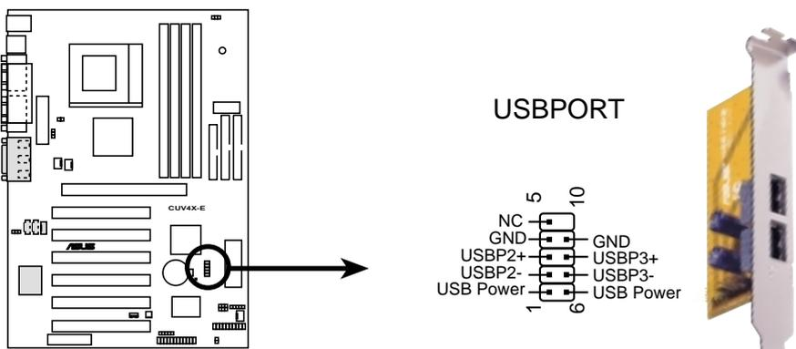
**CUV4X-E Front Panel USB Header**
