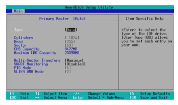
**NOTE:** Before attempting to configure a hard disk drive, make sure you have the configuration information supplied by the manufacturer of the drive. Incorrect settings may cause your system to not recognize the installed hard disk. To allow the BIOS to detect the drive type automatically, select [Auto].
