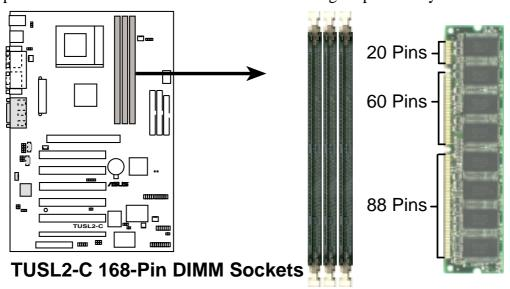
The DIMMs must be 3.3Volt unbuffered SDRAMs. To determine the DIMM type, check the notches on the DIMMs (see figure below).
