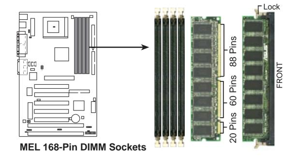
The DIMMs must be **3.3V Unbuffered** for this motherboard. To determine the DIMM type, check the notches on the DIMMs (see figure below).
