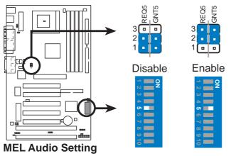
**NOTE:** The onboard audio shares REQ5 and GNT5 with PCI slot 5. Therefore, if the onboard audio is enabled, bus master cards cannot be used on PCI slot 5.
