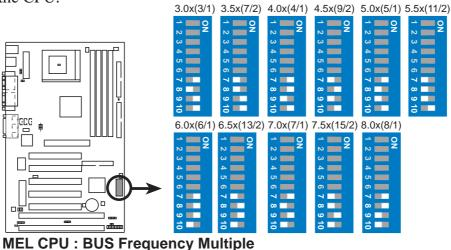
Set the function switches by the Internal speed of your processor as follows:
