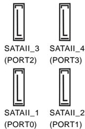
These Serial ATAII (SATAII) connectors support SATAII or SATA hard disk for internal storage devices. The current SATAII interface allows up to 3.0 Gb/s data transfer rate.
