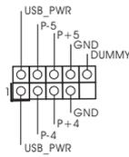
Besides six default USB 2.0 ports on the I/O panel, there is one USB 2.0 header on this motherboard. This USB 2.0 header can support two USB 2.0 ports.
