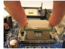
Step 3. Remove PnP Cap (Pick and Place Cap):
