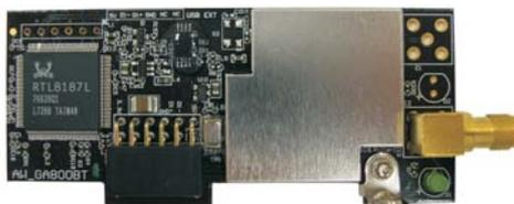
ASRock WiFi-802.11g module is an easy-to-use wireless local area network (WLAN) adapter to support WiFi+AP function. With ASRock WiFi-802.11g module, you can easily create a wireless environment and enjoy the convenience of wireless network connectivity. Therefore, from anywhere within the signal range, you will be able to play LAN games, connect to the internet, access and share printers, and make Internet phone calls easily.
