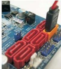
Connect the SATA data cable to the orange SATAII connector (SATAII\_6 (PORT5))
