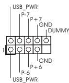
Besides six default USB 2.0 ports on the I/O panel, there are two USB 2.0 headers on this motherboard. Each USB 2.0 header can support two USB 2.0 ports.
