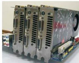
Step 2. Connect the auxiliary power source to the PCI Express graphics card. Please make sure that both power connectors on the PCI Express graphics card are connected. Repeat this step on the three graphics cards.
