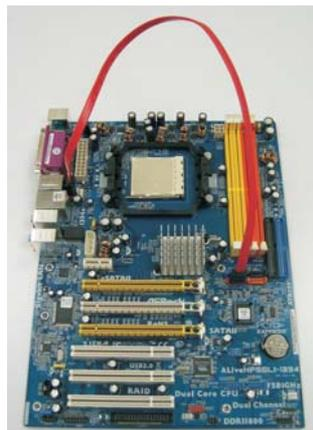
2. Use the eSATAII device cable to connect eSATAII device and the eSATAII port of the I/O shield.
