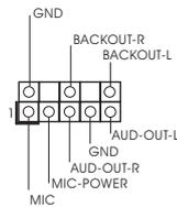
This is an interface for front panel audio cable that allows convenient connection and control of audio devices.
