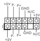
This header can be used to support 2 USB 2.0 ports. It can also be used to support WiFi+AP function with ASRock WiFi-802.11g or WiFi-802.11n module, an easy-to-use wireless local area network (WLAN) adapter. It allows you to create a wireless environment and enjoy the
