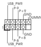
Besides six default USB 2.0 ports on the I/O panel, there are two USB 2.0 headers on this motherboard. Each USB 2.0 header can support two USB 2.0 ports.
