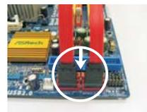
**Step 3** Connect SATA 15-pin power cable connector (Black) end to SATA / SATAII HDD.
