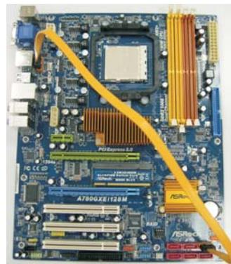
2. Use the eSATAII device cable to connect eSATAII device and the eSATAII port of the I/O shield according to the eSATAII connector that you connect the SATA data cable.
