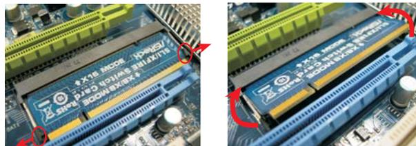
Step 4. Reverse the card direction so as to have the "X8 / X8 MODE" wording side toward the retention slot base. Insert the card into the bottom of the base.
