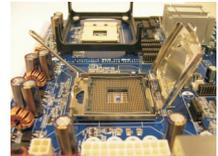
Step 1-3. Rotate the load plate to fully open position at approximately 100 degrees.
