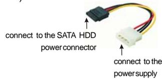
Please connect the black end of SATA power cable to the power connector on the drive. Then connect the white end of SATA power cable to the power connector of the power supply.
