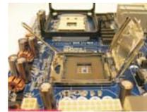
Step 1-3. Rotate the load plate to fully open position at approximately 100 degrees.
