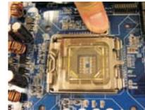
Step 1-2. Rotate the load lever to fully open position at approximately 135 degrees.
