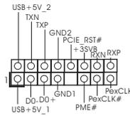
This header supports WiFi+AP function with ASRock WiFi-802.11g or WiFi-802.11n module, an easy-to-use wireless local area network (WLAN) adapter. It allows you to create a wireless environment and enjoy the convenience of wireless network connectivity.
