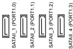
These four Serial ATAII (SATAII) connectors support SATA data cables for internal storage devices. The current SATAII interface allows up to 3.0 Gb/s data transfer rate.
