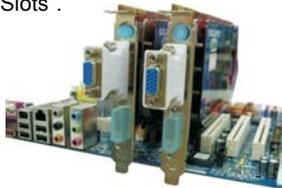
Step 4. Connect two Radeon graphics cards by installing two CrossFire™ Bridge on CrossFire™ Bridge Interconnects on the top of Radeon graphics cards. (CrossFire™ Bridge is provided with the graphics card you purchase, not bundled with this motherboard. Please refer to your graphics card vendor for details.)
