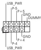
Besides four default USB 2.0 ports on the I/O panel, there is one USB 2.0 header on this motherboard. This USB 2.0 header can support two USB 2.0 ports.
