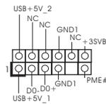
This header supports WiFi+AP function with ASRock WiFi-802.11g or WiFi-802.11n module, an easy-to-use wireless local area network (WLAN) adapter. It allows you to create a wireless environment and enjoy the convenience of wireless network connectivity.
