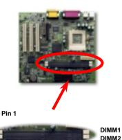
Tip: The driving capability of new generation chipset is limited due to the lack of a memory buffer (to improve performance). This makes DRAM chip count an important factor to take into consideration when you install DIMMs. Unfortunately, there is no way that the BIOS can identify the correct chip count, you need to calculate the chip count by yourself. The simple rule is: By visual inspection, use only DIMMs which are less than 16 chips..
