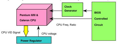
(Automatically generates CPU voltage)
