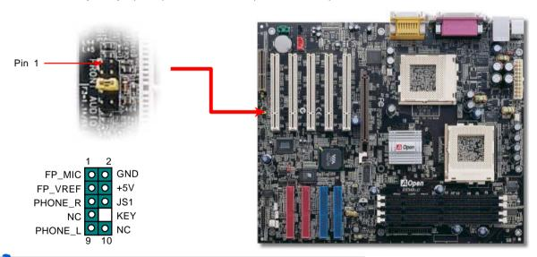
**Note:** Please remove the jumper cap from the Front Panel Audio Connector before you connect the cable. Do not remove this yellow jumper cap if housing without an audio port on the front panel.
