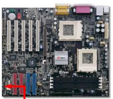
Attach the power LED, speaker, power and reset switch connectors to the corresponding pins. If you enable "Suspend Mode" item in BIOS Setup, the ACPI & Power LED will keep flashing while the system is in suspend mode.
