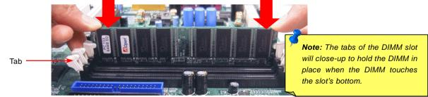
3. Repeat step 2 to finish additional DIMM modules installation.
