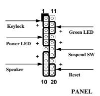
Other housings may have a 12-pin connector. If your housing has this type of connector, connect it to PANEL as shown in the figure. Make sure that the red wire of the connector is connected to +5V.
