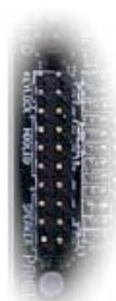
Attach the power LED, speaker, power and reset switch connectors to the corresponding pins. If you enable “Suspend Mode” item in BIOS Setup, the ACPI & Power LED will keep flashing while the system is in suspend mode.
