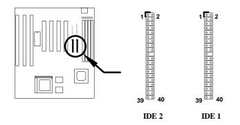
**Caution**: The specification of IDE cable is maximum 46cm (18 inches), make sure your cable does not excess this length.
