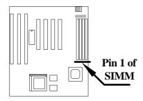
This mainboard has four 72 pin SIMM sockets (Single-in-line Memory Module) that allow you to install system memory from minimum 4MB up to maximum 256MB.
