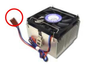
**Note:** You must using 3-pin CPU cooler fan with this motherboard. Only 3-pin cooler fan has support hardware monitoring function.
