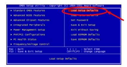
**Warning:** Please avoid of using "Load Turbo Defaults", unless you are sure your system components (CPU, DRAM, HDD, etc.) are good enough for turbo setting.
