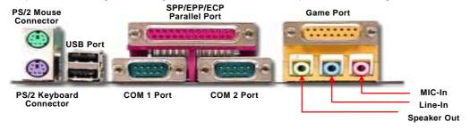
**PS/2 Keyboard:** For standard keyboard, which is using a PS/2 plug.
