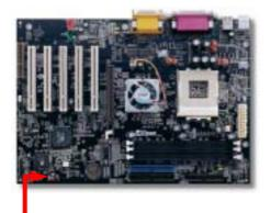
You can clear CMOS to restore system default setting. To clear the CMOS, follow the procedure below.
