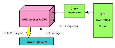
(Automatically generates CPU voltage)
