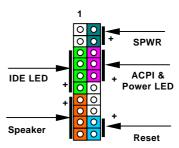
Attach the power LED, Keylock, speaker, and reset switch connectors to the corresponding pins. If you enable "<u>Suspend Mode</u>" item in BIOS Setup, the ACPI & Power LED will keep flashing while the system is in suspend mode.
