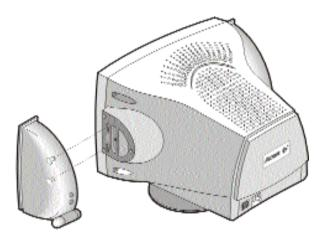
Unlike ordinary speakers, the speakers that came with your Aspire system do not use a power adapter. Instead, it shares power with your system via the PS/2 connector.
