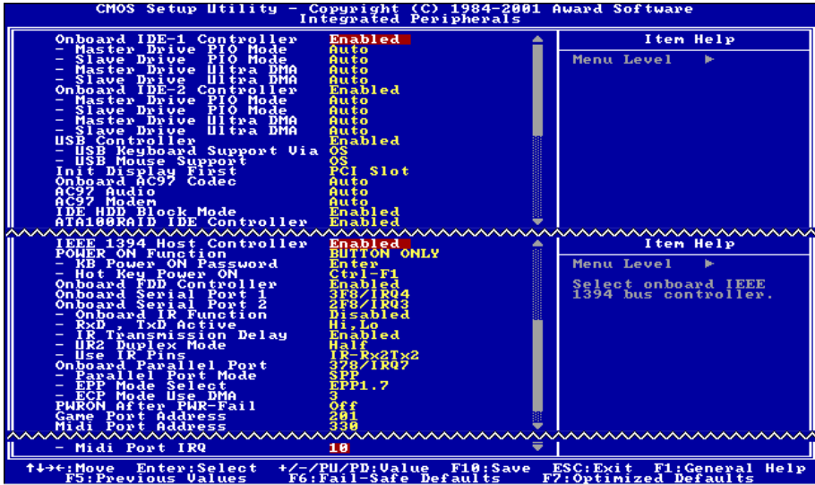
Figure 3-7. Integrated Peripherals Menu Screen
