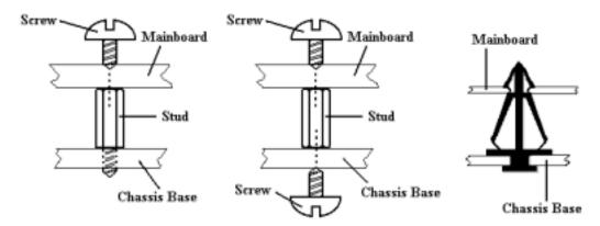
**Note:** If the motherboard has mounting holes, but don't line up with the holes on the base and their are no slots to attach the spacers, don't worry, you can still attach the spacers to the mounting holes. Just cut the button portion of spacers (the spacer may be a little and hard to cut off, so be careful of your hands). In this way you can still attach the motherboard to the base without worrying about short circuits.
