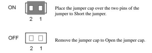
**Note:** To avoid losing jumper caps, attach the removed jumper cap to one of the jumper pins.
