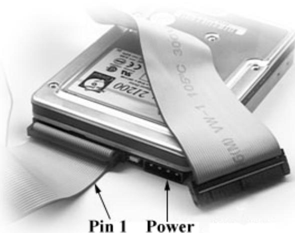
ATA-66 IDE hard drives require a special 80 pin IDE cable which has additional grounding wires. The cable is included in the motherboard package, and is required when using ATA-66 drives. This cable will also support all legacy IDE drives. Note: The blue end of the ATA/66 cable must connect to the motherboard. Some symptoms of incorrectly installed HDDs are:
