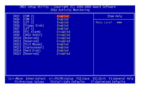
In the screen, you can see a list of IRQs (Interrupt Requests). When an I/O device wants to gain the attention of the Operating System, it asserts an IRQ signal. When the Operating System is ready to respond to the request, it interrupts itself and performs the service. The IRQs Activity Monitoring function monitors the IRQs you select "On". Activity from any of them will awaken a system which has been powered down.
