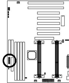
**Pins [3 & 5] Turbo LED switch** - The Turbo function is not supported by this mainboard. Therefore, the Turbo LED will always remain lit as long as the system power is on.
