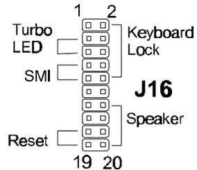
**Pins [17 & 19] Reset switch lead** - Connects to the Reset Switch lead from the system's case. The reset switch is used to "cold-boot" the system without actually turning off the power, reducing wear and tear on the power supply.
