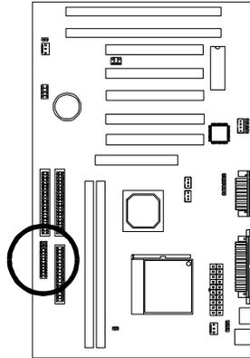
**Pins [3 & 5] Turbo LED switch** - The Turbo function is not supported by this mainboard. Therefore, the Turbo LED will always remain lit as long as the system power is on.
