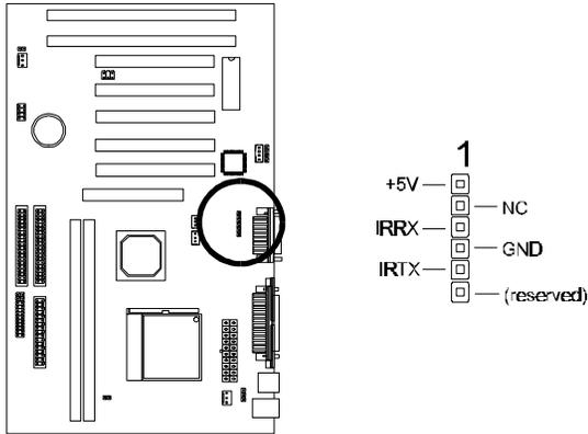
The IrDA connector bracket hooks directly to this connector on the mainboard. This connector provides support for the optional wireless transmitting and receiving infrared module. You must first configure through “UART2 Mode” in ***INTEGRATED PERIPHERALS SETUP*** where UART2 is directed, COM2 or IrDA.
