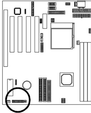
**Pins [7 & 9] SMI suspend switch lead** - If your system's case has a suspend switch, hook the lead from the switch to pins 7 & 9. A suspend switch is used to save electricity by putting the system into a suspend mode when the computer is not being used. For this switch to be functional, "*Suspend Mode*" must first be enabled in the **Power Management Setup** in the BIOS Setup utility.
