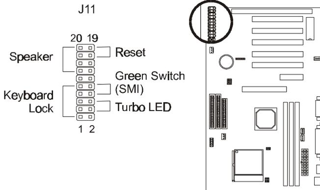
**Pins [3 & 5] Turbo LED lead** – The Turbo function is not supported by this mainboard. Therefore, the Turbo LED will always remain lit as long as the system power is on.
