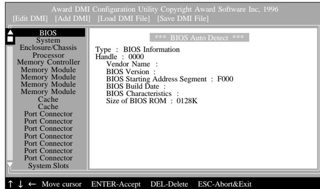
The four menus located on top of the DMI Configuration Utility screen are Edit DMI, Add DMI, Load DMI File and Save DMI File. Use the ← or → (left or right) arrow keys to select a menu from the Menu bar.
