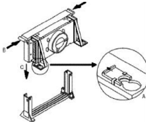
5. Slide the clips on the supports (A) forward until they click into place to hold the pegs securely. (Apply slight pressure on the peg and push the peg toward the clip while pushing the clip forward.) Push the latches on the processor (B) outward until they click into place in the Retention Mechanism. The latches must be secured for proper electrical connection of the processor.
