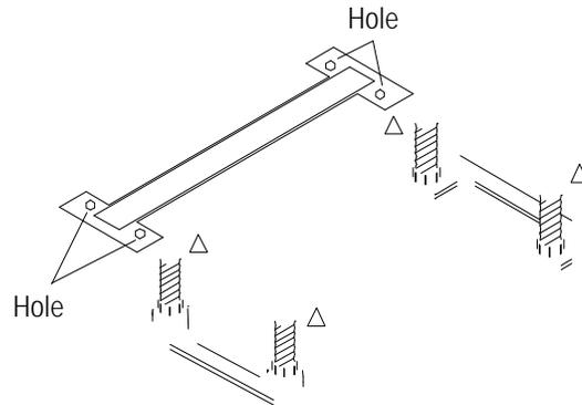
3. Hold the Retention Mechanism upright and position it above the processor slot.
