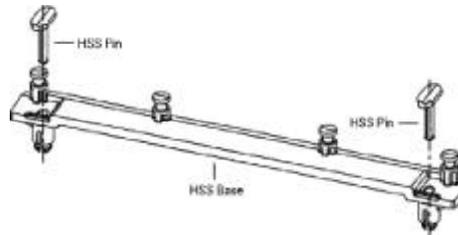
4. Install the HSS Base by pushing each side down firmly into the holes on the system board. (The HSS Base can only be installed in one direction). Make sure it locks into place.
