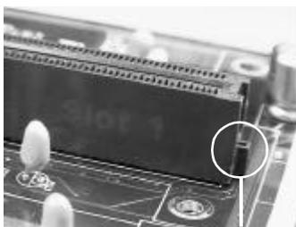
**Pentium II Slot Connector and Key Pin**
