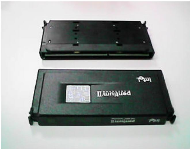
Figure 2:OEM Pentium® II Processor
