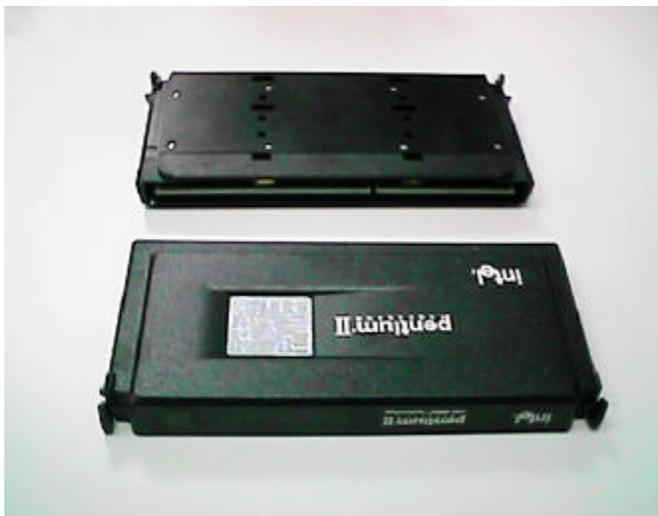
Figure 2:OEM Pentium® II Processor
