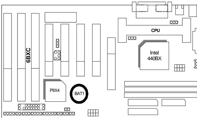
**Danger of explosion if battery is incorrectly replaced.**
