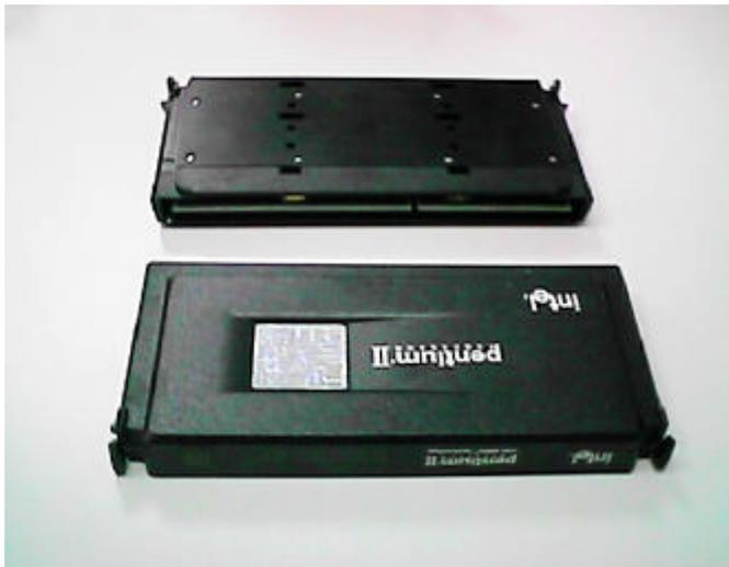
Figure 2:OEM Pentium® II Processor
