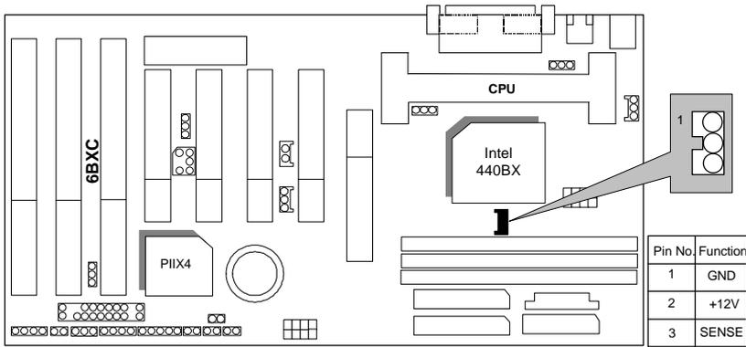
System FAN : System Fan Power Connector
