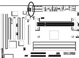
Use the Sony compatible cable enclosed with your CD-ROM disk drive to connect the CD-ROM to your mainboard. This will enable your CD-ROM's audio function.
