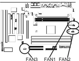
These added connectors allow the fan to draw their power from the mainboard instead of the disk drive connector. The board's management extension hardware is able to detect the CPU and system fan speed in rpm (revolutions per minute). These connectors supports 3-pin cooling fans with minimum of 3500 RPM. The wiring and plug may vary depending on the manufacturer. On standard fans, the red is positive (+12V), the black is ground, and the yellow wire is the rotation signal.
