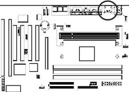
If you want to use a USB keyboard, you must enable the USB keyboard support function in BIOS's Integrated Peripherals menu (See Section 3-7). USB is an open industry standard, providing a simple and inexpensive way to connect up to 125 devices to a single computer port. Keyboards, mice, tablets, digitizers, scanners, bar-code readers, modems, printers and many more can all be used at the same time.
