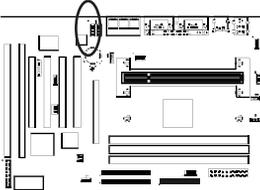
Use the cable enclosed with your CD-ROM disk drive to connect the CD-ROM to your mainboard. This will enable your CD-ROM's audio function.
