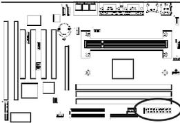
This mainboard requires a power supply of at least 200 watts. **The power cord leading from the system's power supply to the external power source must be the very last part connected when assembling a system.**
