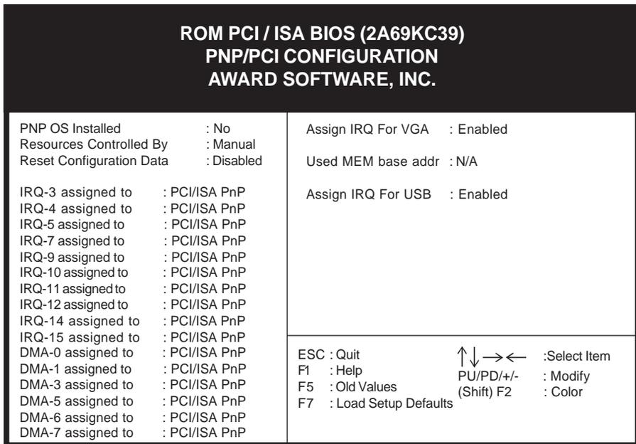
Figure 3-7 PCI & ONBOARD I/O Setup Screen
