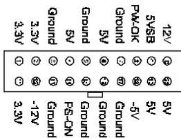
The ATX power supply provides a single 20-pin connector interface which incorporates standard +/-5V, +/-12V, optional 3.3V and Soft-power signals. The Soft-power signal, a 5V trickle supply is continuously supplied when AC power is available. When the system is in the Soft-Off mode, this trickle supply maintains the system in its minimum power state.
