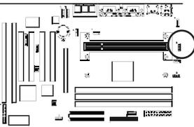
This board supports the chassis instruction monitoring feature of the management extension hardware by means of a mechanical or photo sensor switch attached to the motherboard through this 1x3-pin chassis security header. The mechanical switch is set to open for normal computer operation.
