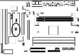
The SB-LINK serves as a bridge between the mainboard and Creative's PCI sound card. This connector delivers Sound Blaster 16 compatibility for real-mode DOS games.
