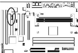
If you enable the COM2 Mode in BIOS's Integrated Peripherals menu the COM2 port will support IR functions. (See section 3-7)
