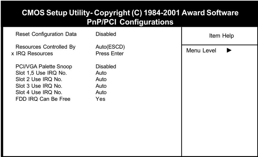
**Figure 3-7 PnP/PCI Configurations Screen**
