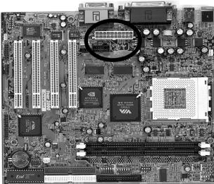
The power cord leading from the system's power supply to the external power source must be the very last part connected when assembling a system.
