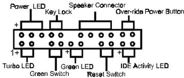
When the Soft-OFF by PWR-BTTN function is enabled, pushing the power button rapidly will switch the system to Suspend mode. Any occurrence of external activities such as pressing a key on the keyboard or moving the mouse will bring the system back to Full-On. Pushing the button while in Full-On mode for more than 4 seconds will switch the system completely off. See Over-ride Power Button Operation diagram.
