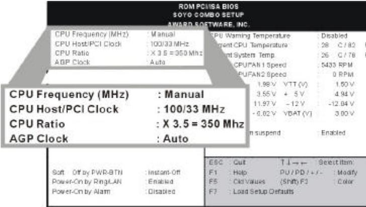
Available [CPU Speed] settings on your SY-6IBM Motherboard are detailed in the following table. If you set this field to [Manual], you are then required to fill in the next two consecutive fields: (1) the CPU Ratio, and (2) the CPU Frequency.
