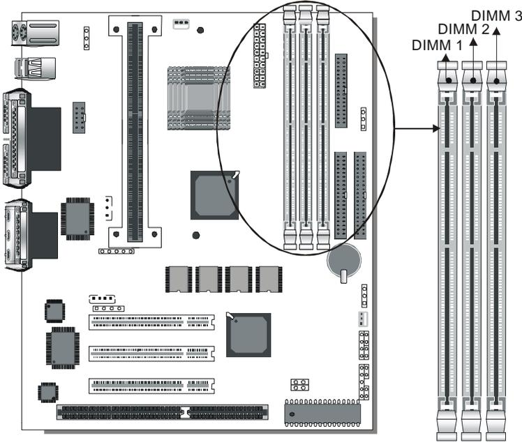
his motherboard features 3 x DIMM Banks for 168-pin 3.3V unbuffered and registered DIMM modules, providing support for up to 768MB of main memory using DIMM modules from 8MB to 256MB. For 66MHz front side bus CPUs use 12ns or faster memory; for 100MHz front side bus CPUs use 8ns (100MHz, PC100 compliant) memory.
