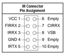
There are two ways to use this IR function. One is to connect a 5-pin IR device and treat it like an ordinary IR port. The other way is to connect a 10-pin IR device and use the advanced "IR Wake Up" PC function. Ask your IR provider for the new "IR Wake Up" function.
