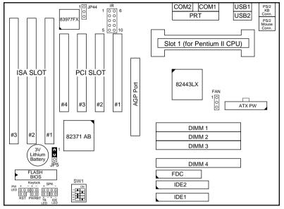
Figure 1–2. Mainboard Default Setting
