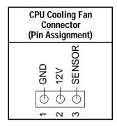
Note: Make sure the pin assignment of our CPU Cooling Fan is matched with this connector before connecting it, otherwise, you may damage either the mainboard or the cooling fan.
