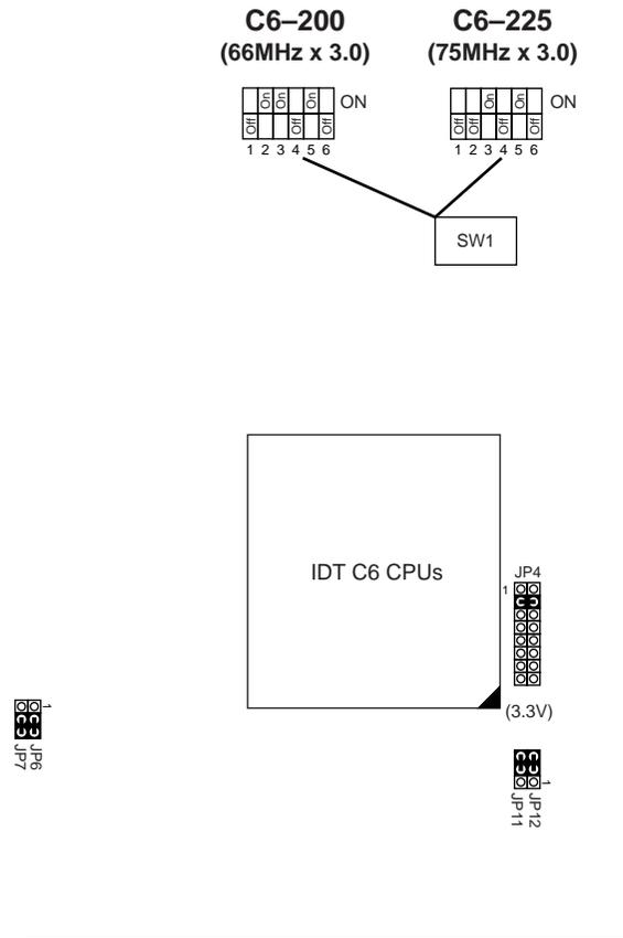
Figure 2-5. CPU Type Configuration
