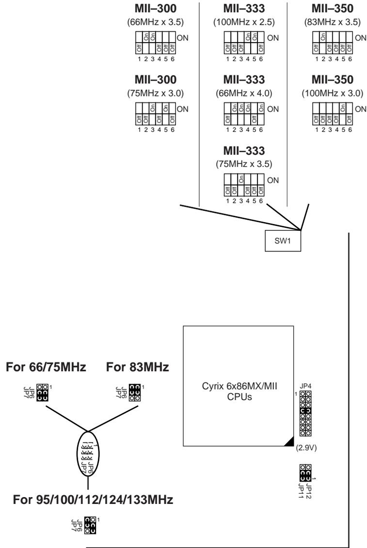
Figure 2-4. CPU Type Configuration
