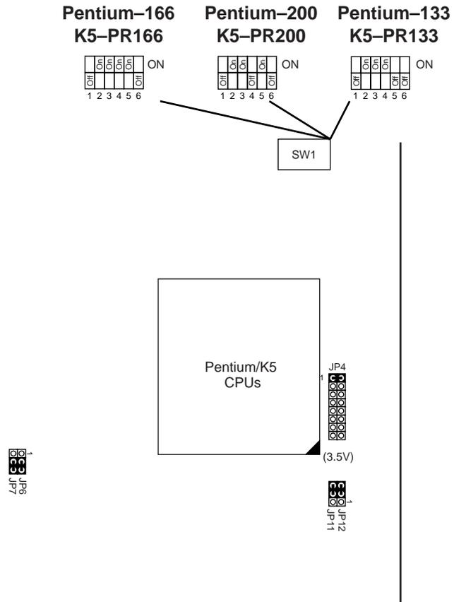
Figure 2-6. CPU Type Configuration
