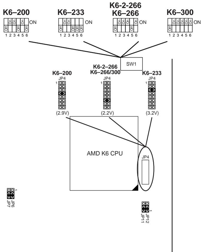
Figure 2-2. CPU Type Configuration
