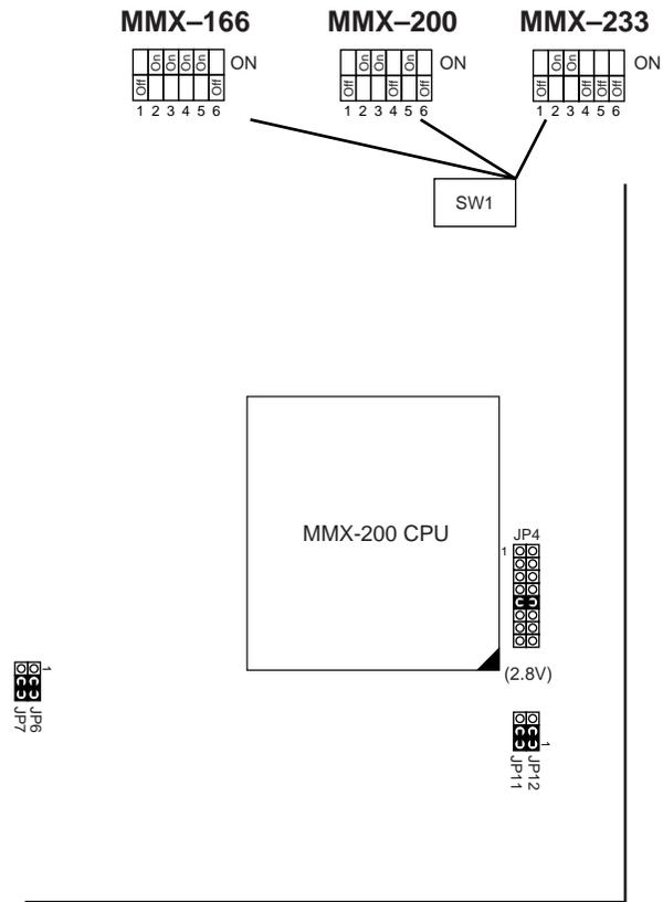
Figure 2-1. CPU Type Configuration
