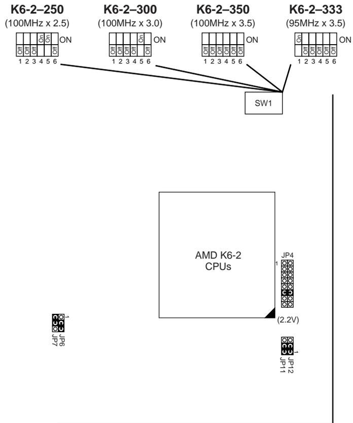
Figure 2-3. CPU Type Configuration
