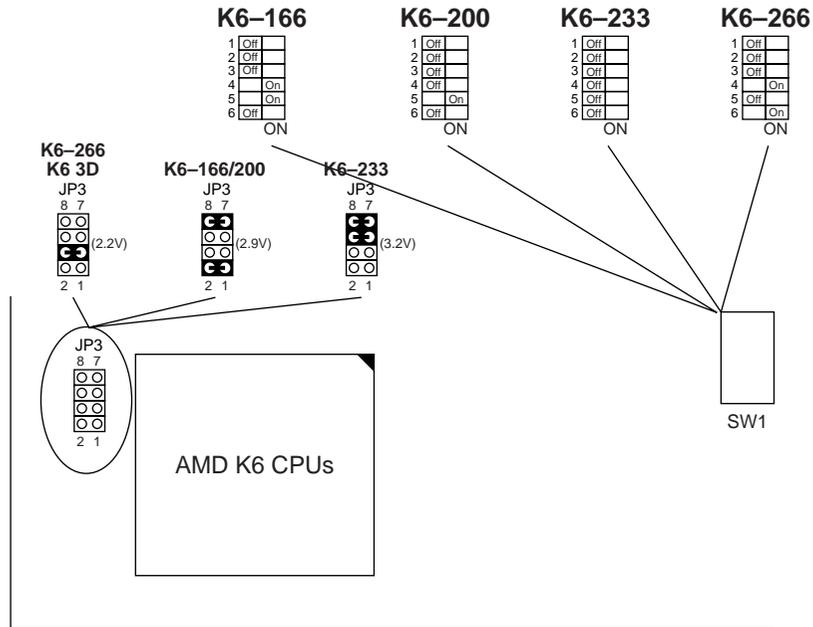
Figure 2-2. CPU Type Configuration
