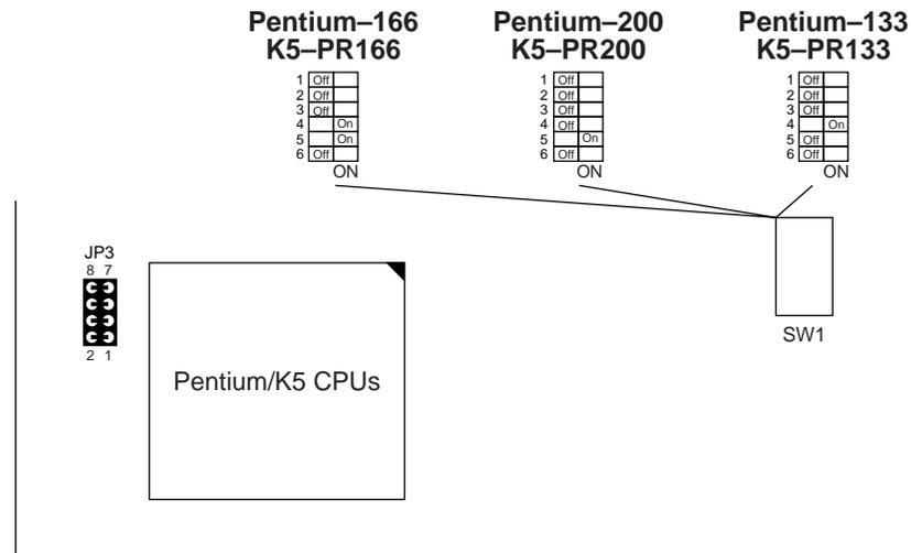
Figure 2-6. CPU Type Configuration
