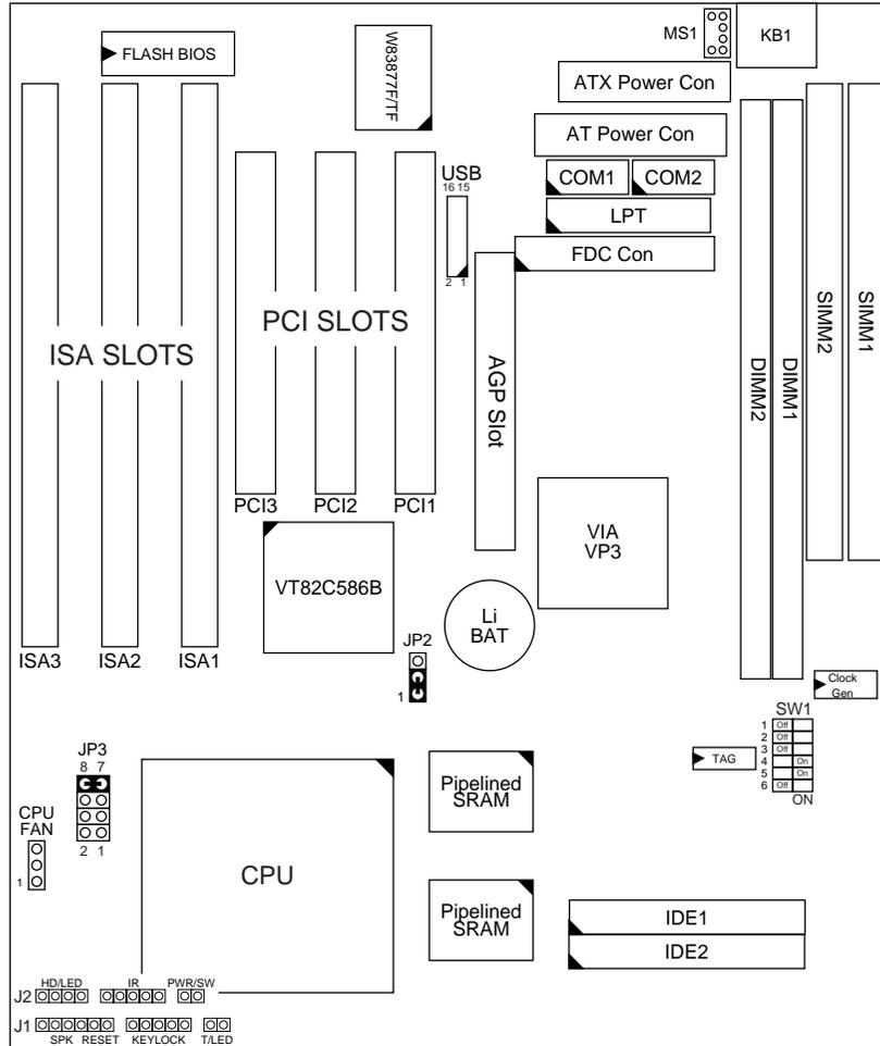
Figure 1-1. SL-54T5 Motherboard Layout
