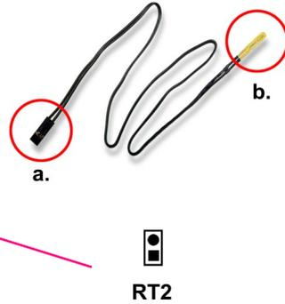
We provide a thermal cable in the mainboard package. This thermal cable is to monitor device which will generates a lot of heat, such as HDD, Graphics card etc. Please connect one end of the thermal cable (A) to mainboard RT2 header, and tape the other end of thermal cable (B) on to the device which you want to monitor. After you finish the thermal cable installation, you will **see the detected temperature in BIOS setup or Hardware monitor utility.**
