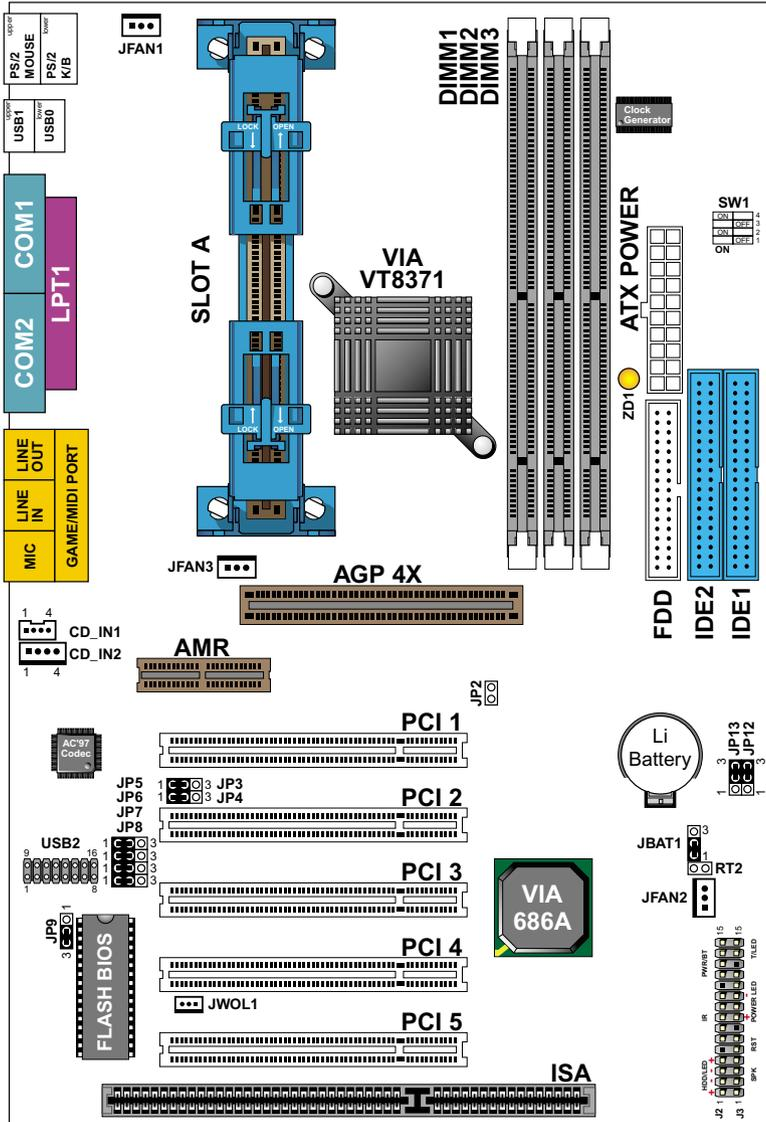
**NOTE:** Under 100MHz / 133MHz FSB, the SDRAM spec must complaint PC-100 / PC-133 spec.
