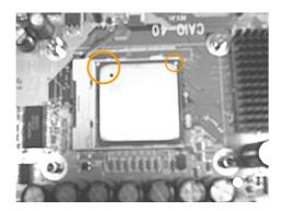
Step  ${\bf 3}$ : Push the lever down to close the socket.
