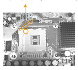
Step 2 : Insert the CPU into the socket. Please keep the lever angle when inserting CPU.
