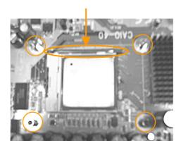
Step 4 : Attach the heat sink onto the CPU. Be careful not to scrape the motherboard when mounting a clamp CPU fan or else damage may occur to the motherboard.
