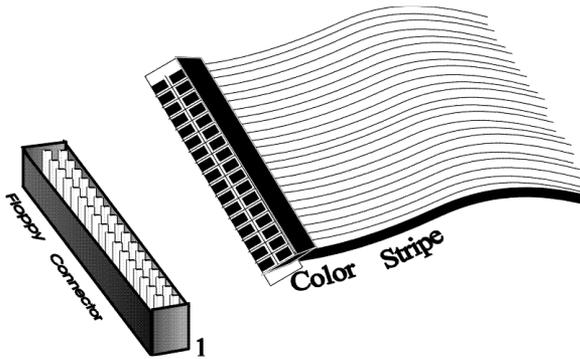
The motherboard supports up to two 720 KB, 1.44 MB, or 2.88 MB 3½" drives and 360 KB and 1.2 MB 5¼" drives. The connecting cable is a 34-pin ribbon connector with two 34-pin edge connectors for attaching the floppy disk drives. There is a small twist in the cable between the floppy connectors. The last (end) connector should be connected to floppy drive A: as shown below.
