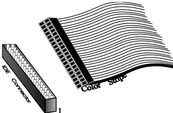
J10 is a 40-pin dual-inline shrouded connector that connects an ATA IDE drive to the primary onboard IDE connector. This motherboard supports IDE Mode 0 and LBA (Logical Block Address) mode, high capacity drives (over 528 MB), 32-bit data transfer, and fast IDE transfer. These IDE features are configured in Peripheral Setup in the AMIBIOS Setup utility. Disable the onboard IDE interface in Peripheral Setup to use an ISA ESDI, RLL, MFM, or SCSI hard disk drive.
